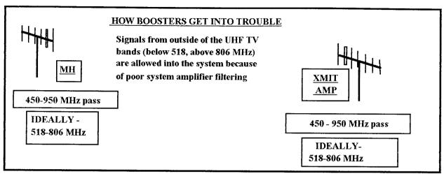
you need to see a visual display of all of the signals passing through the system to be certain the trap(s) you are installing are operating <u>after</u> installation on the correct frequency, and, there are not other undesired frequencies getting through the system as well.
